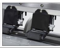
**6.Press roller**The adjustable pressure roller is more convenient to use.
