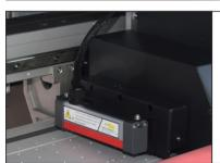
**3.Static eliminator** Effectively avoid the interference of static electricity on the printing of the nozzle and improve the printing accuracy.
